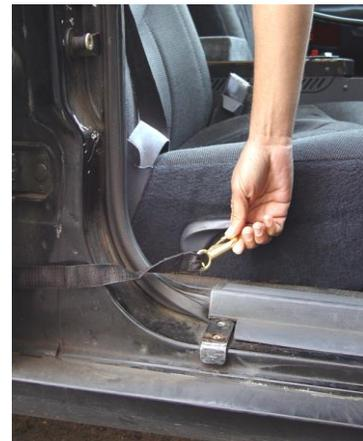
**No portion of the strap should be exposed outside of the vehicle.**
