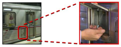
Open emergency door cover plate and pull handle down to release the door latch. Pulling the emergency door release handle will activate the emergency brake lock preventing the train from moving. The doors can then be manually pulled open.
